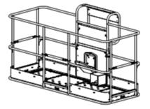
▲ Tri-entry platform with two sliding mid-rails and center mounted swing gate
