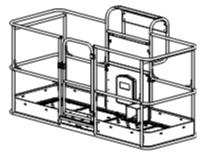
A Tri-entry platform with three sliding mid-rails
